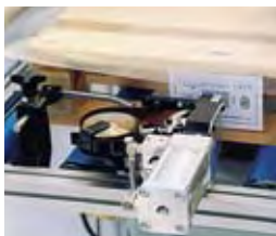
Labelling station: One or two stapling heads nailing labels onto the pallet base.
