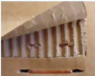
Blind stapling: staple is bent within the carton layers.
