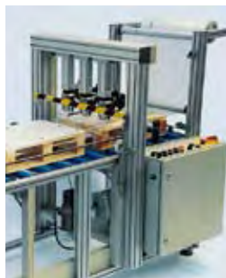
Nailing station with stapling heads C 13-30/80. Foils or carton are nailed fully automatically onto wooden pallets. The feed travel up to 80 mm compensates different pallet heights. The staple is pressed into the material which avoids any damage like cutting through the film or cardboard.
